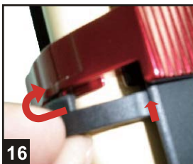
16 Slide the "C" slots of the Q/R locking lever safety onto matching parts of Q/R locking mount. Then snap the hook to lock onto the Q/R locking lever.
