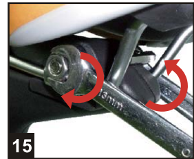
15 Tighten with 13mm spanner. Do not over tighten, ( 250-350 kgf.cm / 25-35 Nm )
