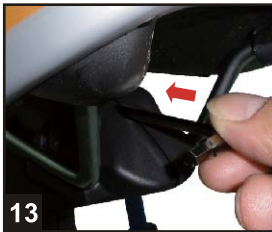
13 Put the Allen key into its mounting hole.
