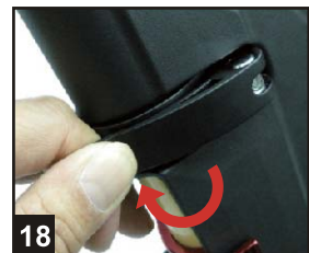
18 Make sure the Q/R lever is correctly adjusted and lock closed.
