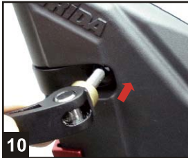
10 Fit the Q/R clamp and lever from Left.
