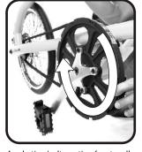
Apply the belt on the front pulley.
