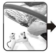
Press the belt in the freewheel while you apply the new 18" rear wheel.
