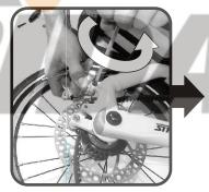
Loosen 1x part number 340-04-15 and rotate part nr. 340-05 around the loose 340-04-15 part.
