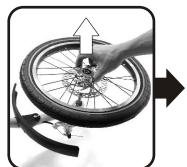
Rotate part nr. 240-05 around the loose 240-04-15 part and pull of the front wheel after you have removed 375.
