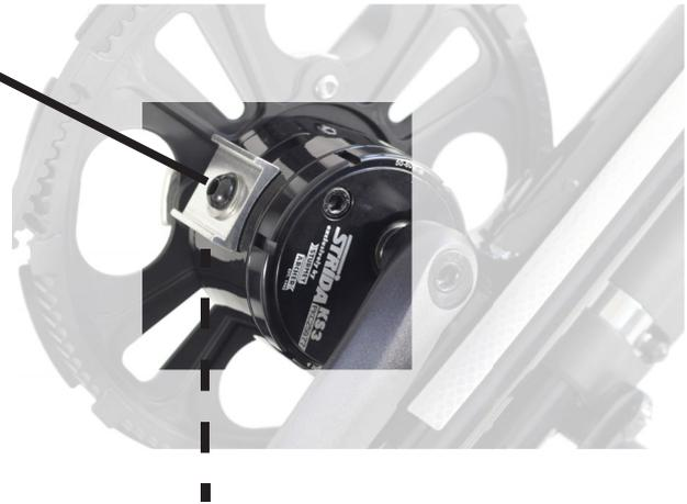
Below the alloy part, you will see a toothed blocking element for the KS3 gearbox. This should remain in place, with the alloy element (3) on top of that.
