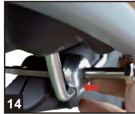
14 Put the saddle screw with clip in from the right side.
