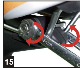
15 Tighten with 13mm spanner. Do not over tighten. ( 250-350 kgf.cm / 25-35 Nm )
