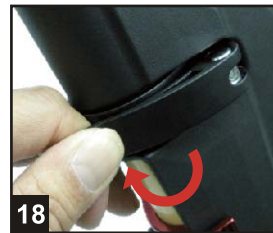
18 Make sure the Q/R lever is correctly adjusted and lock closed.
